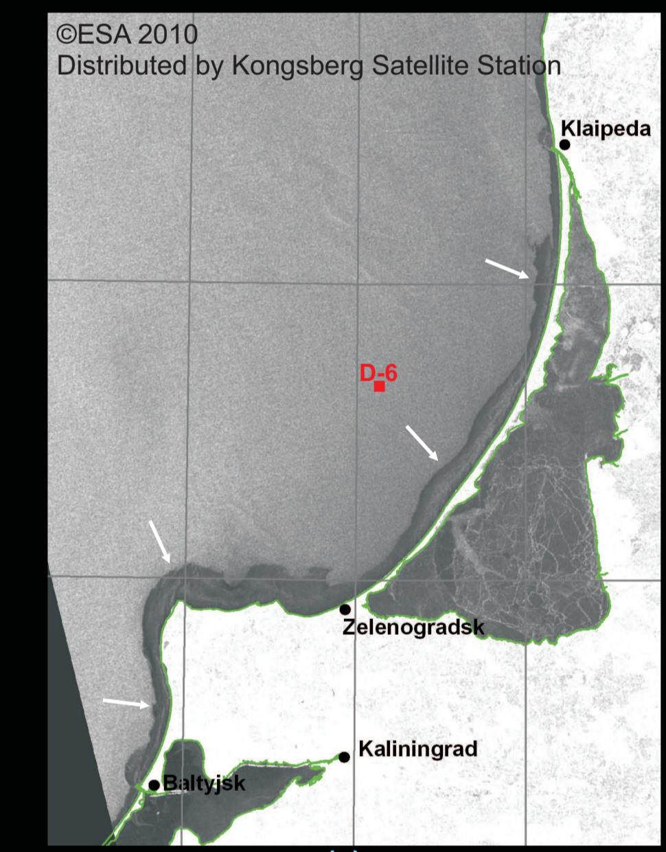
Grease ice spreading on 31.01.2010. a) Radar image from ENVISAT (20:05 UTC). Grease ice along the shore is shown by blue arrows. b) Picture taken from the shore near Zelenogradsk.
